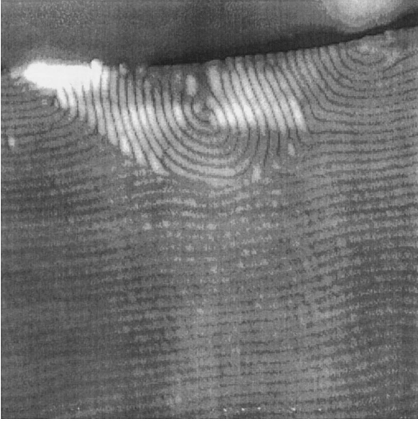
FIG. 7. An AFM image of a microtome cut, oblique to the free surface. The image shows a cut through a focal conic domain, embedded in the planar bulk texture (image length 7000 nm).
